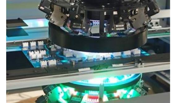
550 BTL with top & bottom cameras, for double sided inspection at the same time.
