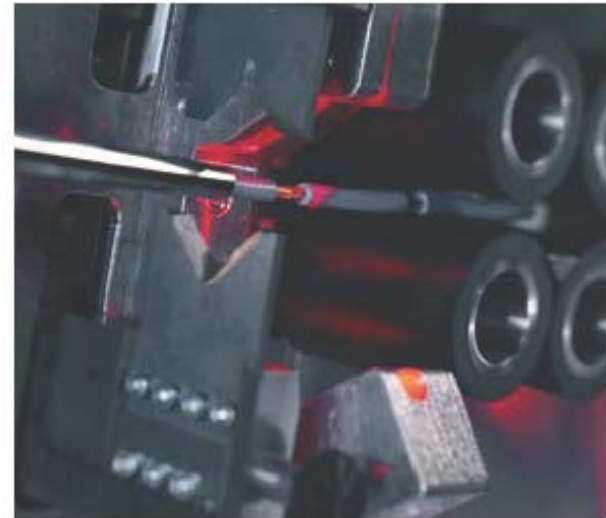
Komax Kappa 310 – Laser Sensor
