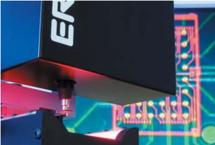
ERSA IR/PL 550 – placement head in the foreground. With a view of the software controlled alignment in the background
